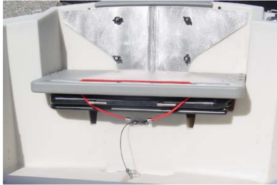
Rear seat with rudder and standard leeboards underneath
