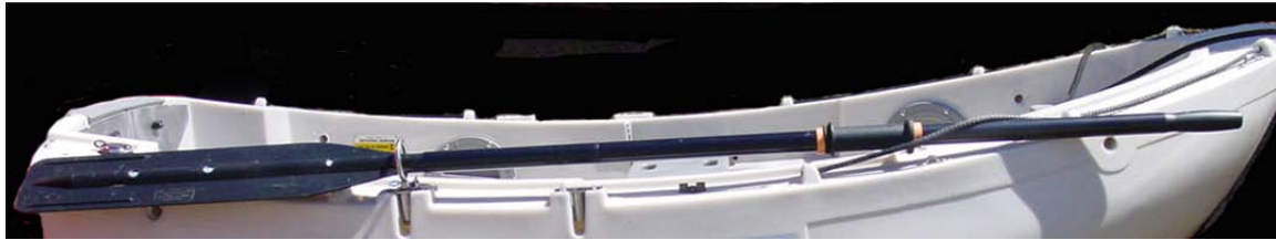
Oars shipped in locked position (see Method A. Setting the Oarlocks to Allow Locking the Oars when Shipped, above)
