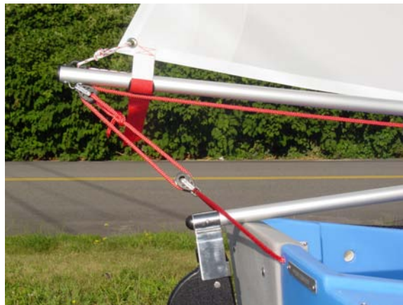
Step G, completed. Traveler installed on boat
