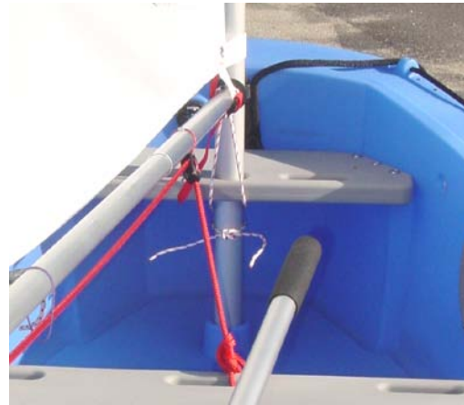
Step H. Mast installed in boat
