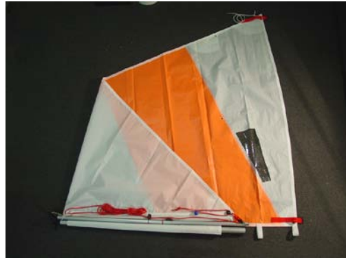
Step E-3. Fold boom up alongside mast
