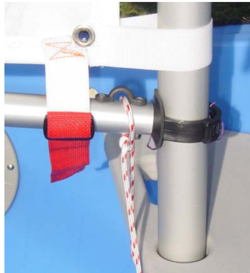
Step H-5. Downhaul passed through the boom's pad-eye. Boom snapped to mast
