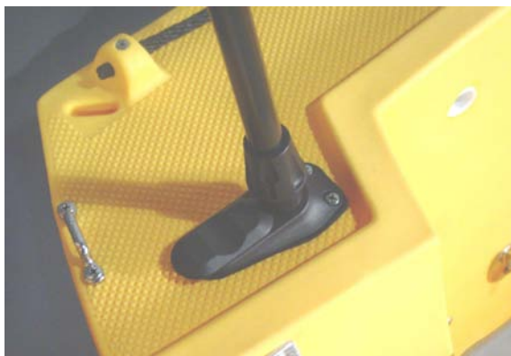
Pole light base (locked in place)
