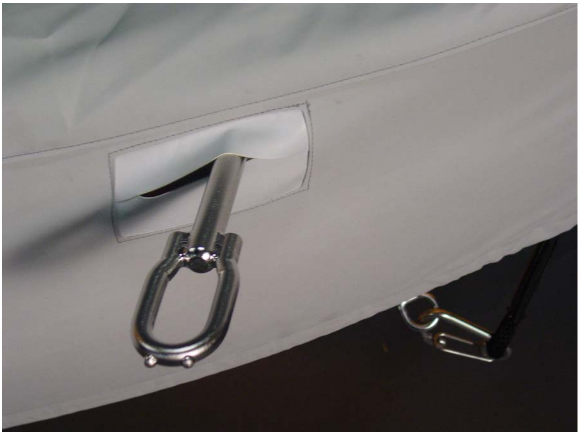
Detail of boat cover for Weaver davits, showing one of four openings in sides for davit loops
